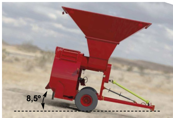
Figure 4 - Bagging machine parked pointing down a slope
